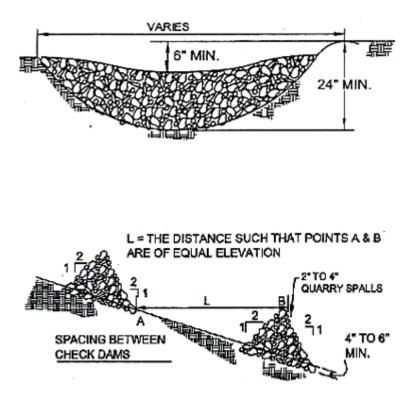
Figure 8 – Rock Check dams (temporary or permanent)
