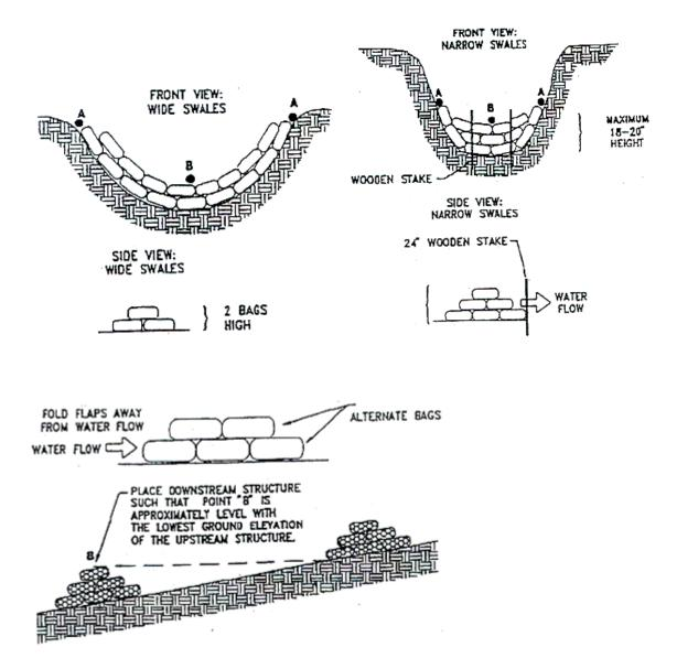
Figure 7 - Sand Bag Check Dams (temporary)
