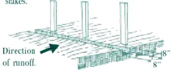
3) If the filter fabric did not come attached to the posts, staple the filter material to the posts. Extend the fabric into the trench.
