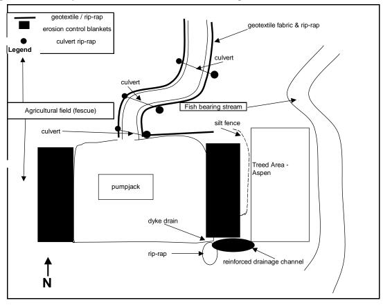
Figure 19 - Site Map - Erosion and Sediment Control Mitigation Plan
