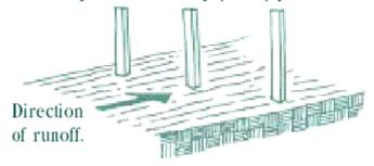
2) Excavate a 8" x 8" trench upslope along the line of stakes.
