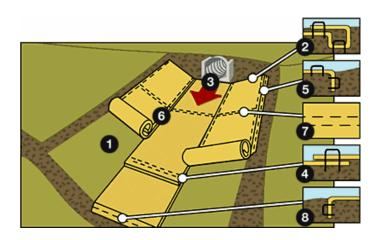
Figure 5 - Installation of Erosion Control Blanket on a slope and in a drainage channel
