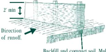
Backfill and compact soil. Make sure the fabric is covered by the compacted soil to avoid gaps.
